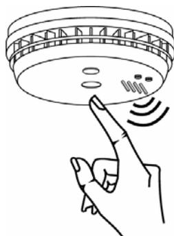
**Figure B- 20: Testing the Smoke Alarm**
