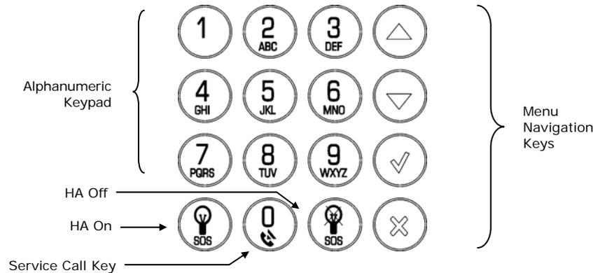
Figure 4-1: On-board Keypad Layout
