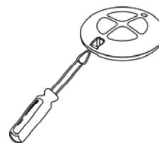
Figure B- 23: Opening the EL-2714's Casing
