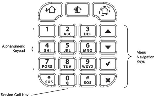
Figure 4-1: On-Board Keypad Layout
