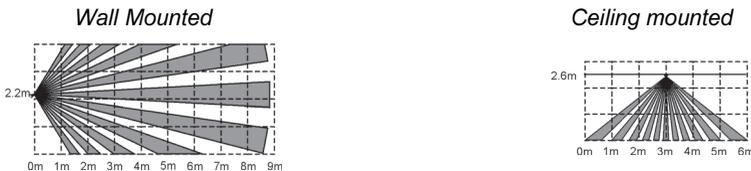
**Figure B- 10: Lens Coverage Pattern (Side View)**
