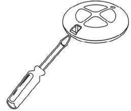
Figure B-33: Opening the EL-2714's Casing
